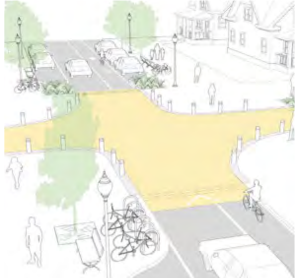
Raised Intersection / Traffic Calming
